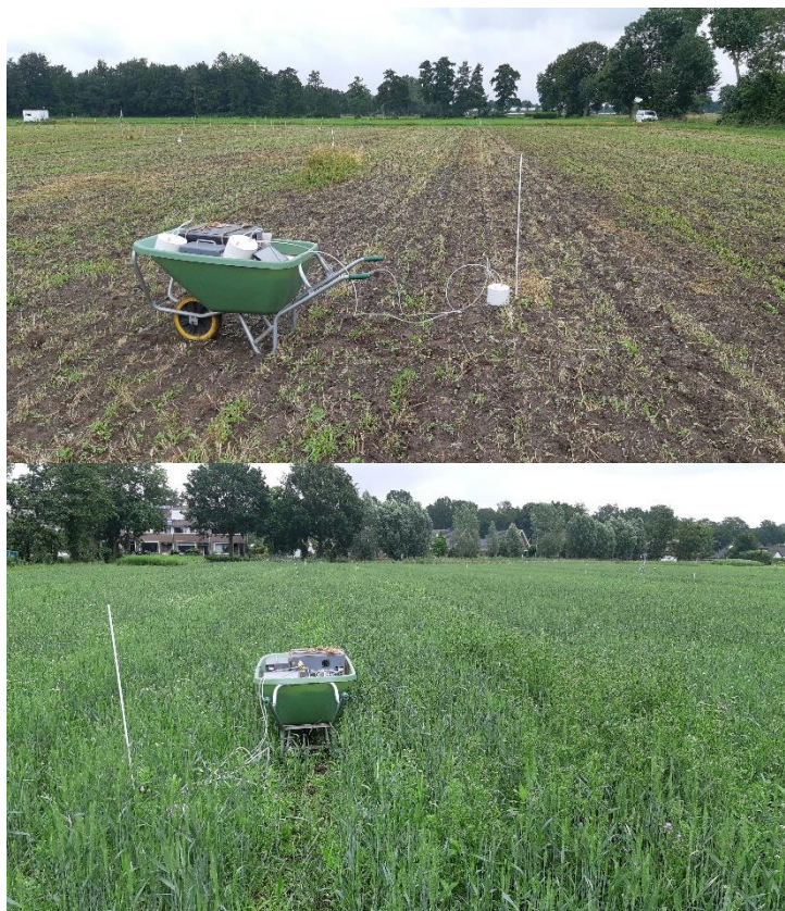
Figure 6: Static chamber measurements on reseeded (upper figure) and wheat (lower figure).
