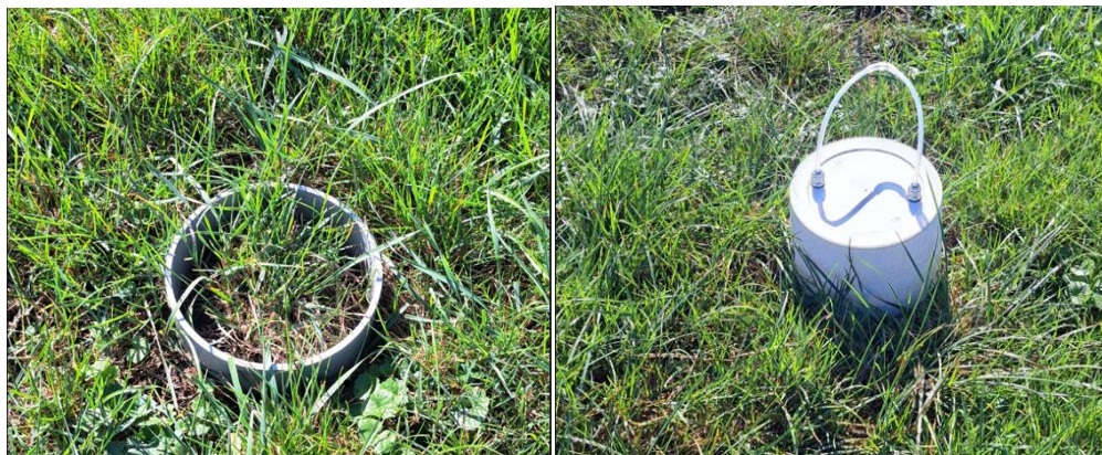
Figure 4: Installed pvc collar as a base of the chamber measurements (figure left) and a gas-tight chamber on top of the collar (figure right).
